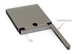
Swivel open the locking bar and then lift the tab vertically.
