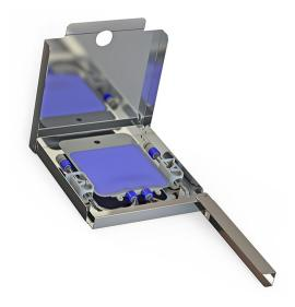
Place filled, Aramus bag into cassette. Orient any connected tubing, clamps, and connectors as shown to fit into the cassette. Ensure no components are raised above the cassette's side walls.
