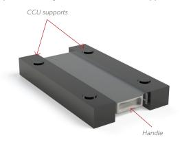
CCUs are used to facilitate controlled freezing. When freezing in standard static or blast freezers, insert CCU onto the long sides of the RoSS shell, one at a time. The CCU should fit snuggly with the shell.
