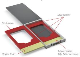
Remove only the upper tubing foam and the rod foam before placing the bag inside.
