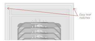
Figure 3. Easy tear notches
