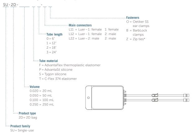
Notes: Assemblies sold sterilized. Assembly temperature performance is component-dependent. Assemblies are individually double-bagged.
