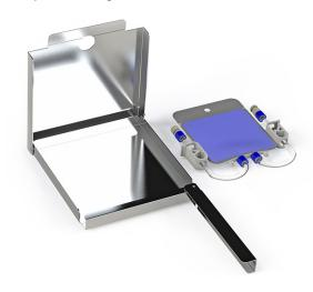
Inspect the cassette assembly to ensure no damage or significant bulging occurred during freezing. The locking bar and tab should be secure.
